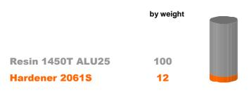
**WARNING:** The mixing ratio must be accurately followed. It is not possible to change the ratio, it would result in lower mechanical properties. The mixture should be thoroughly stirred to ensure full homogeneity. It is important to note that epoxy systems tend to heat up much faster in a pot than as a thin film. It is therefore necessary to only mix the necessary amount usable within the given pot life. Keeping the mixture in flat open containers reduces the risks of exothermic reaction.
