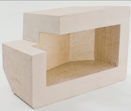
Cast block with removable core and taper of mould
